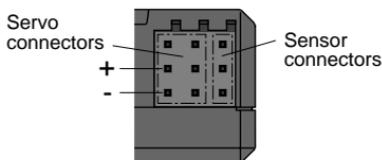
When a battery is connected to the servo connectors, the control amp is activated.
