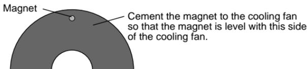
If the cooling fan is unbalanced and vibrates, etc., balance it by mounting the spare magnet to the opposite side of the cooling fan in the opposite polarity (so that it does not output a signal).
