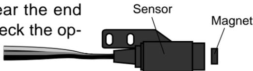
This is the side at which the displayed value increases. Install the magnet with this side facing the sensor. Mark this side of the magnet with a felt tip pen.
