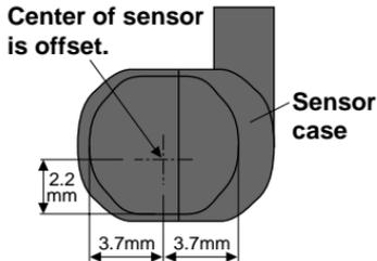
Align the sensor center position and the center of the magnet shown in the figure at the left.
