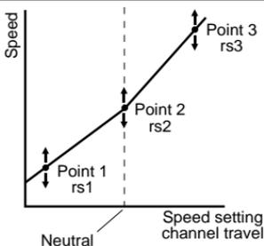
The speed changes linearly on a line connecting points 1, 2, and 3.
